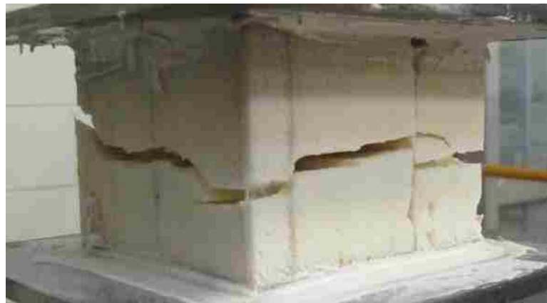
Figure 4.21: Damage During Core Failure for Flatwise Tension Testing on Type 2
