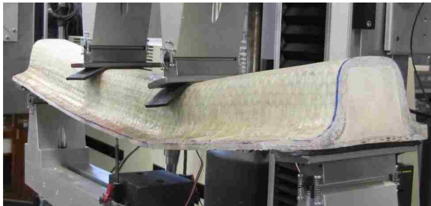
Figure 5.38: Four Point Flexural Testing Ultimate Failure Due to Compression Failure of the Top Facing Under the Load Point for Type 3
