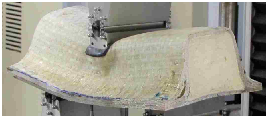
Figure 5.17: Three Point Flexural Testing Ultimate Failure by Excessive Local Indentation and Fracturing of the Shear Layers for Type 3
