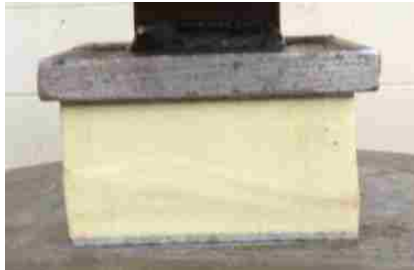
Figure 4.8: Damage at Failure for Flatwise Compression Testing on Type 1
