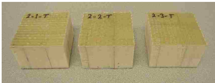
Figure 4.14: Flatwise Tension Testing Specimens for Type 2
