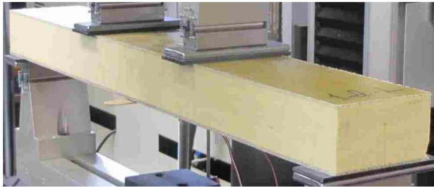
Figure 5.19: Four Point Flexural Test Specimen for Type 1
