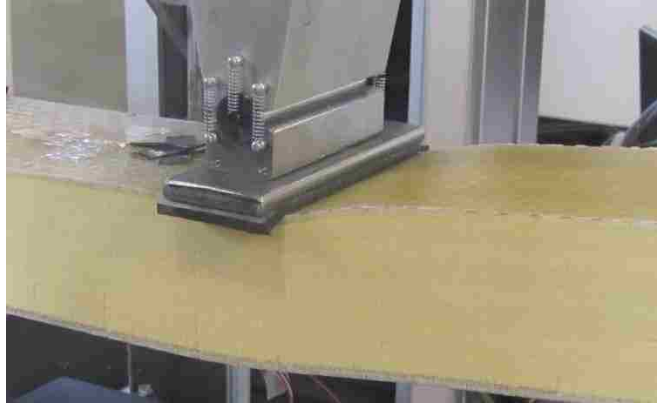
Figure 5.26: Four Point Flexural Testing Initial Failure Due to Local Indentation for Type 1
