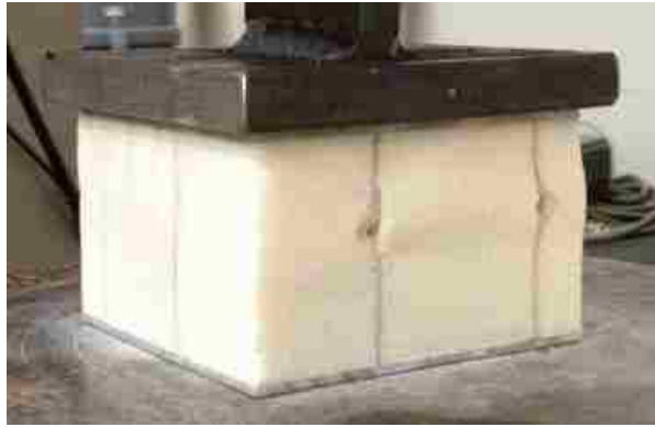
Figure 4.11: Damage at Failure for Flatwise Compression Testing on Type 2
